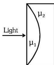
Equivalent focal length is given by  $\frac{1}{f_{eq}} = \frac{1}{f_1} + \frac{1}{f_2}$
